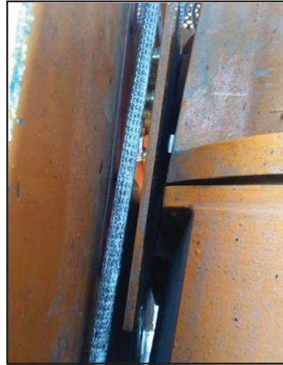
Figure 2: Bolts that have come loose or failed, causing the motor junction box to slip on the TESCO EXI-600 Top Drive
