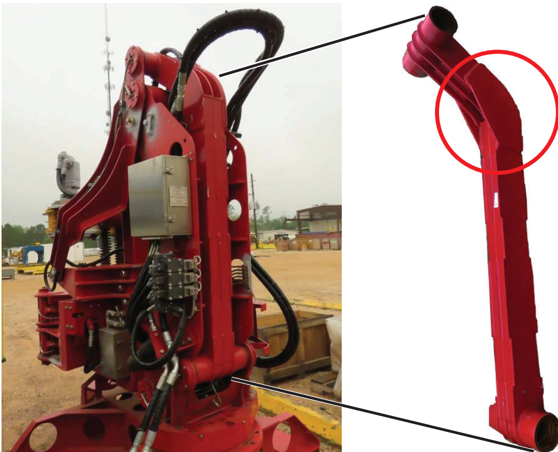
Figure 1: Inspect the entire TM80 Tie Bar for cracks in the weld or material, especially the indicated area. Contact RigLine 24/7™ Support immediately if cracks are found.
